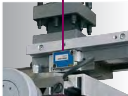
· Magnetic tape with active sensor
