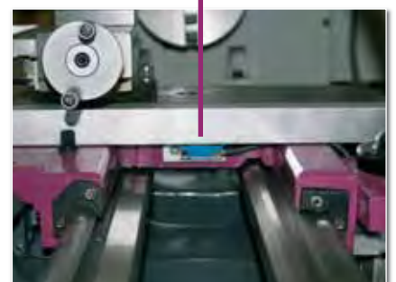
· Magnetic tape with active sensor
